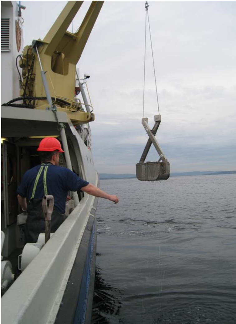
Figure 8 Collection of sediment samples using a van Veen grab.
